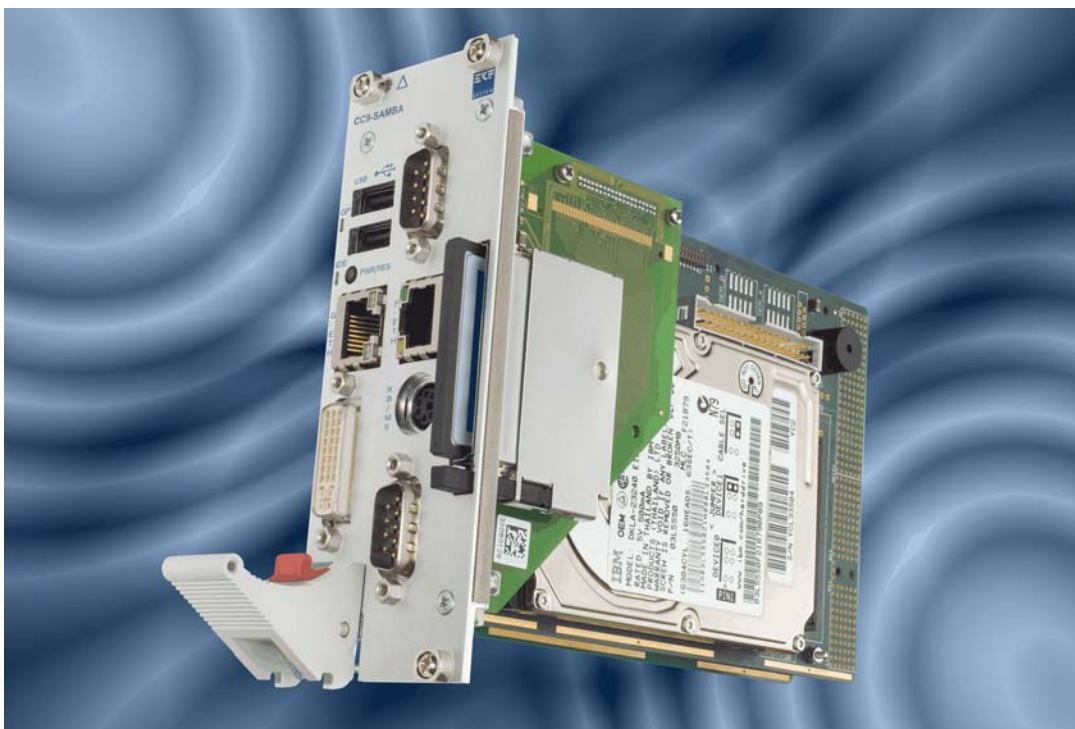
Front Panel CF Card Slot on Top of the CCB-2-BOSSANOVA
